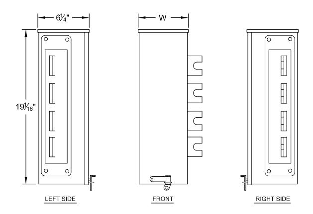
BUSSED SPACERS ARE USED WHEN ADDITIONAL SPACE IS REQUIRED BETWEEN ADJACENT ENCLOSURES TO ALLOW HINGED DOORS TO OPEN OR FOR UTILITY REQUIRED METER CLEARANCE.
